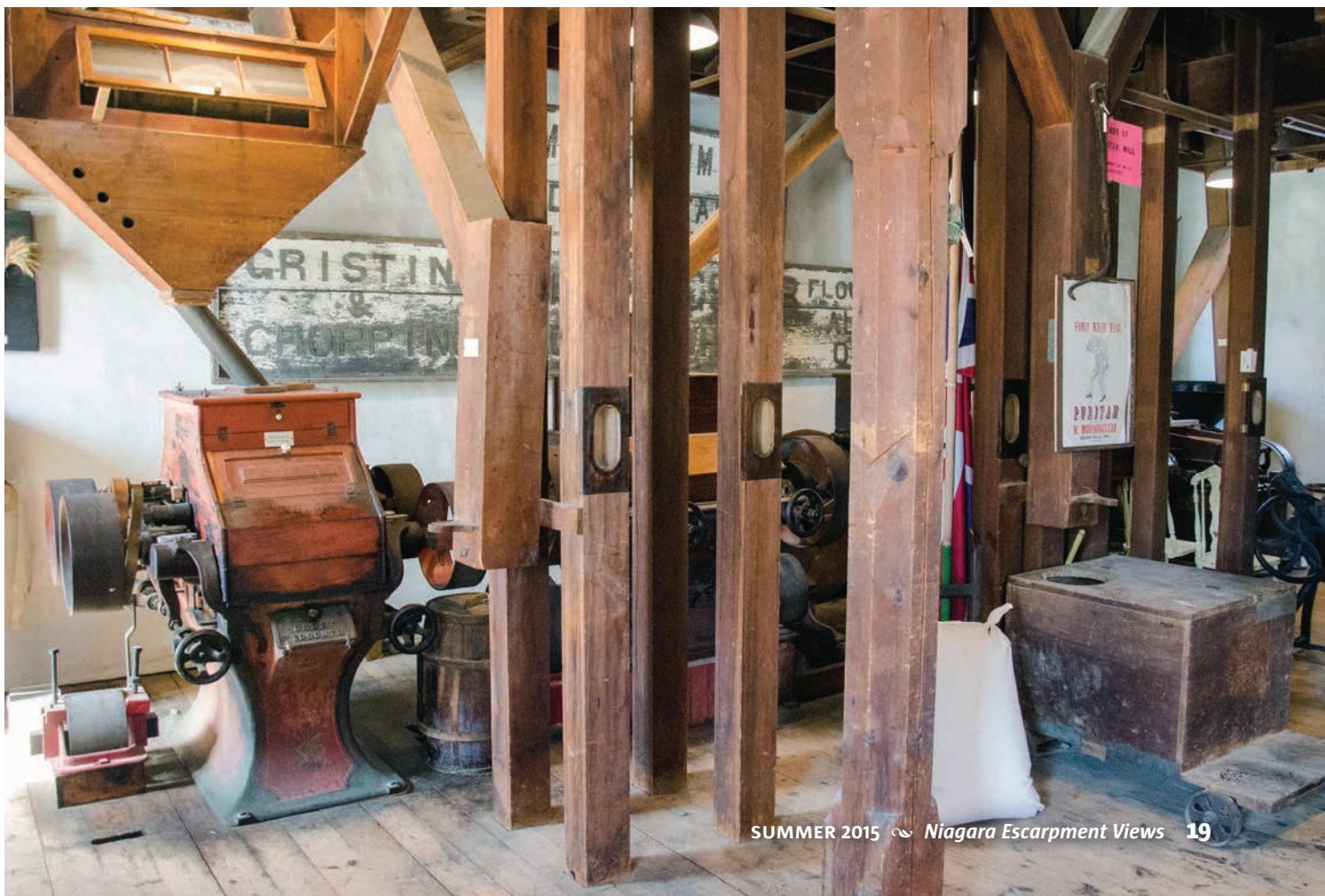
▼ Interior of Mill showing roller milling equipment and grain elevators, part of the 1893 industrial process.
